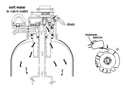
During FAST RINSE, the rotor & disc is positioned so water flow enters the resin tank through the top distributor, and exits through the bottom distributor, to the drain.
